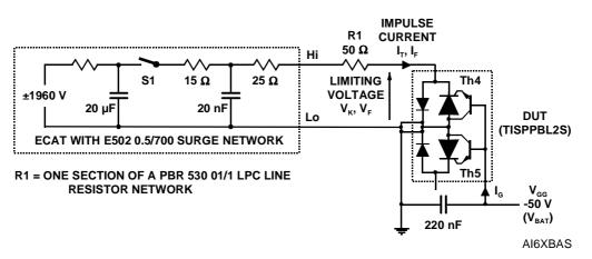
Figure 3. TEST CIRCUIT FOR MEASUREMENT OF LIMITING VOLTAGE
