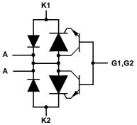
Terminals K1, K2 and A correspond to the alternative line designators of T, R and G or A, B and C. The negative protection voltage is controlled by the voltage,  $V_{GG}$ , applied to the G terminal. SD6XAP
