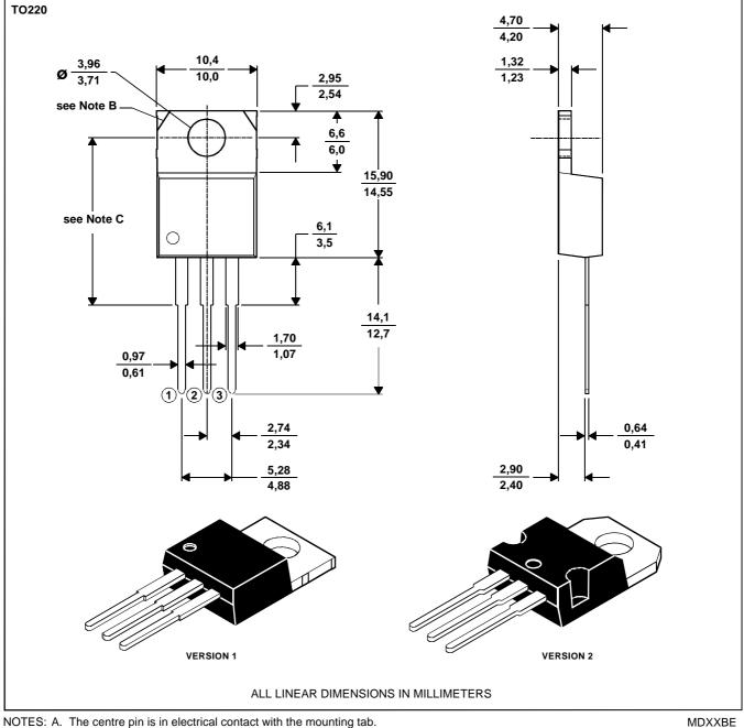
B. Mounting tab corner profile according to package version.
