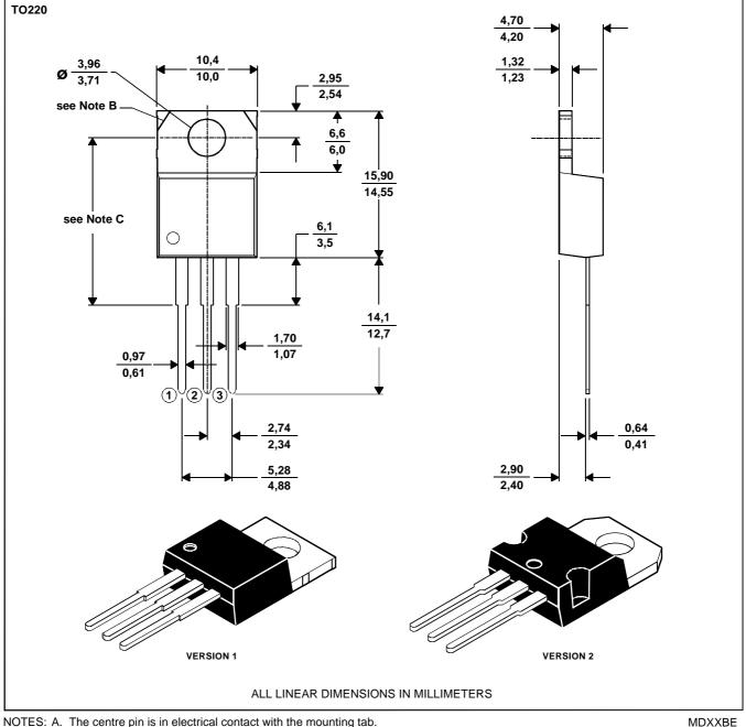
B. Mounting tab corner profile according to package version.
