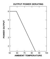
Typical Performance: (Tc=25°C, Vin=Nom VDC, Rated Load)
