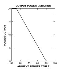
Typical Performance: (Tc=25°C, Vin=Nom VDC, Rated Load)
