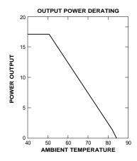
Typical Performance: (Tc=25°C, Vin=Nom VDC, Rated Load)
