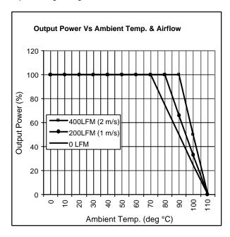
The 9-36V and 18-75V input voltage versions of this series feature a 4:1 input voltage range and can achieve operation at full power at 85°C ambient temperature with only convection cooling.
