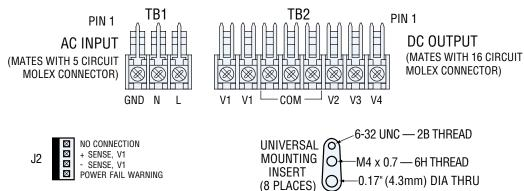
INPUT & OUTPUT CONNECTIONS: 6-32 SCREW WIRE CLAMPS ON 0.312" (7.9mm) CENTERS, 0.045" (1.1mm)
