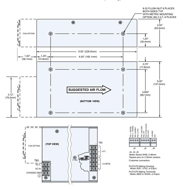
INPUT & OUTPUT CONNECTIONS: 6-32 SCREW TERMINAL ON 0.375" (9.5mm) CENTERS
