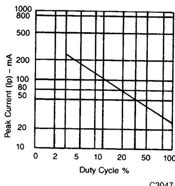
Fig. 5. Max Peak Current vs. Duty Cycle %
