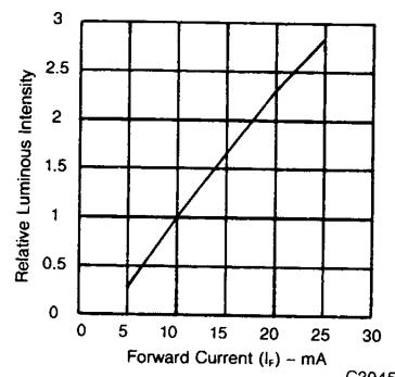
Fig. 3. Relative Luminous Intensity vs.
