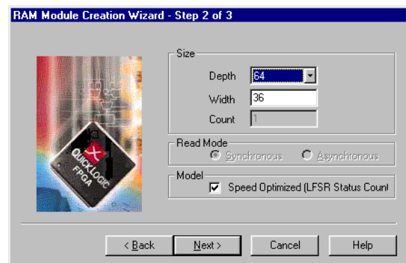
FIGURE 2. Graphical Interface to create FIFO
