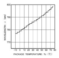
Fig. 4 Dependence of wavelength on temperature
