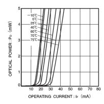
Fig. 1 Optical output vs. operating current
