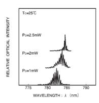
Fig. 5 Dependence of emission spectrum on optical output
