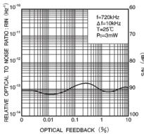
Fig. 8 Dependence of noise on optical feedback
