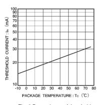
Fig. 2 Dependence of threshold current on temperature
