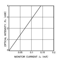
Fig. 6 Monitor current vs. optical output
