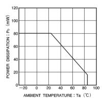
Fig.3 Power dissipation vs. ambient temperature
