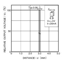
Fig.8 Relative output voltage vs. distance
