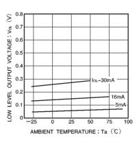
Fig.5 Low level output voltage vs. ambient temperature
