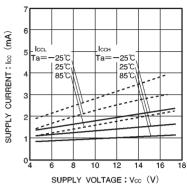
Fig.6 Supply current vs. supply voltage
