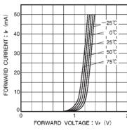
Fig.2 Forward current vs. forward voltage
