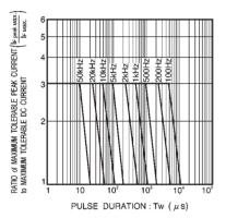
Fig. 6 Maximum tolerable peak current vs. pulse duration
