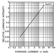
Fig. 23 Luminous intensity vs. forward current
