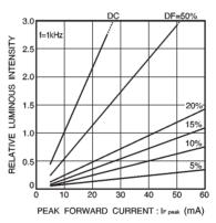
Fig. 25 Luminous intensity vs. peak forward current
