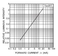
Fig. 11 Luminous intensity vs. forward current
