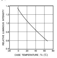
Fig. 10 Luminous intensity vs. case temperature
