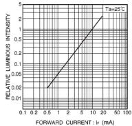
Fig. 5 Luminous intensity vs. forward current
