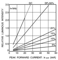
Fig. 19 Luminous intensity vs. peak forward current
