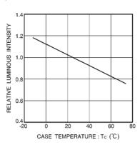
Fig. 22 Luminous intensity vs. case temperature
