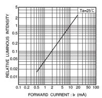
Fig. 17 Luminous intensity vs. forward current
