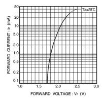
Fig. 21 Forward current vs. forward voltage
