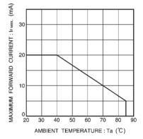
Fig. 20 Maximum forward current vs. ambient temperature
