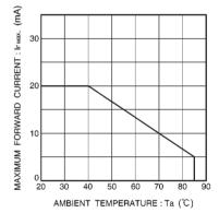
Fig. 8 Maximum forward current vs. ambient temperature
