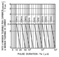
Fig. 24 Maximum tolerable peak current vs. pulse duration
