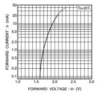
Fig. 9 Forward current vs. forward voltage
