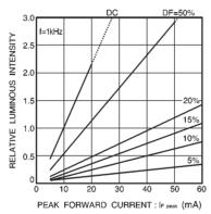
Fig. 7 Luminous intensity vs. peak forward current
