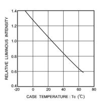
Fig. 4 Luminous intensity vs. case temperature
