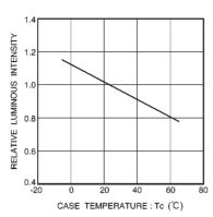
Fig. 16 Luminous intensity vs. case temperature
