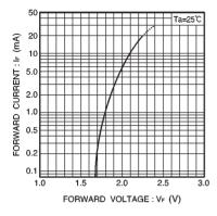
Fig. 15 Forward current vs. forward voltage
