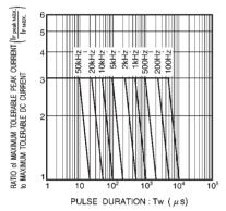
Fig. 12 Maximum tolerable peak current vs. pulse duration
