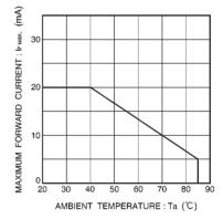
Fig. 14 Maximum forward current vs. ambient temperature
