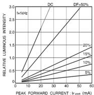
Fig. 13 Luminous intensity vs. peak forward current
