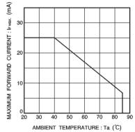
Fig. 26 Maximum forward current vs. ambient temperature
