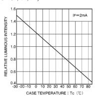
Fig. 3 Luminous intensity vs. case temperature
