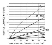
Fig. 4 Luminous intensity vs. peak forward current
