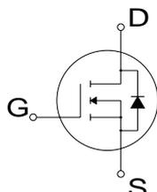
StarMOS is a new generation of high voltage N-Channel enhancement mode power MOSFETs. This new technology minimises the JFET effect, increases packing density and reduces the on-resistance. StarMOS also achieves faster switching speeds through optimised gate layout.
