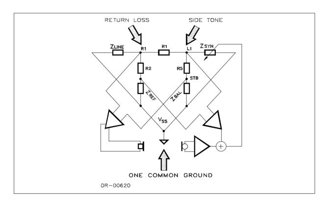
Side Tone is controlled along with Return Loss by a Double Balance Bridge as shown in Fig. 1.
