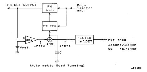
The FM detection filter (gyrator) is controlled at 4.5 MHz by the control current (Iref1) generated by reference circuit 1. At the same time, precision control is performed by using the control current (Iref2) derived by detecting the offset from the detected output so that the FM detector phase relationship is  $90^{\circ}$ . As a result, automatic control makes an ideal quadrature detector possible.
