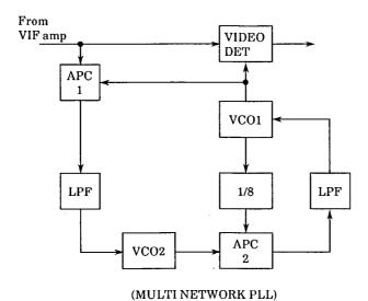
The multinetwork PLL has two VCO circuits. Each of these form a separate PLL. The operational relationship between these circuits is as follows:
