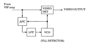
In these blocks, if the VCO coil is not adjusted to the IF frequency, a phase difference will appear in the control loop. As a result, the PLL detector detection axis will shift from the ideal  $180^{\circ}$ . The group delay, DP characteristics, etc., deteriorate as a result.
