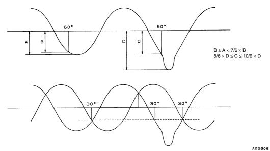
Note: Note that the intersections between the special magnetization and general waveforms and the intersections between pairs of general waveforms must be set up to be 30° apart.
