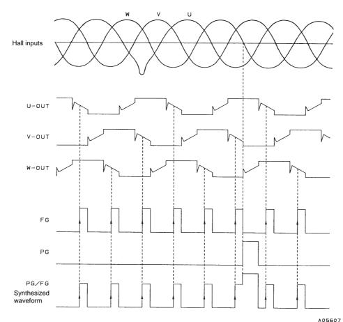
Note: The Hall inputs are defined as follows:  $U = U_{IN}1 - U_{IN}2$ ,  $V = V_{IN}1 - V_{IN}2$ , and  $W = W_{IN}1 - W_{IN}2$ . Inputs to the Hall input pins must be applied in the phase order shown in the timing chart.
