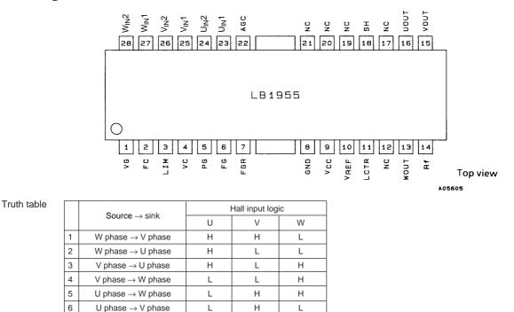
Note: The Hall input "H" and "L" values are defined as follows: "H" means that for that phase the (+) input is higher than the (-) input, and "L" means that for that phase the (+) input is lower than the (-) input. However, note that an input potential difference corresponding to the Hall to output gain is required.
