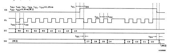
Note: 1. The data conversion time varies with the value of the pull-up resistor, since the DO pin is an n-channel open drain circuit.
