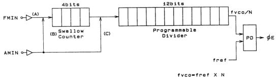
Figure 7 Programmable Divider
