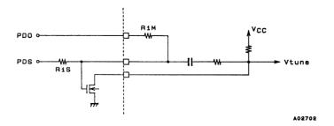
Figure 10 Charge Pump Connections
