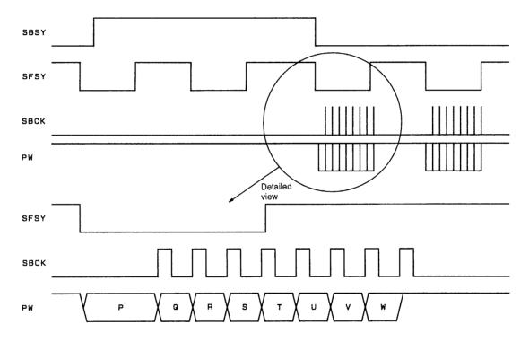
The timing of the rise and fall of the SFSY signal is converted into that shown in the figure below according to the timing of the start bit in the user bits in the input data.
