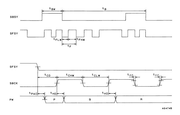
The LC8904Q subcode interface uses the user bit subcode sync word and start bit for system timing extraction. Therefore, since SBSY and SFSY will change with that timing, user bit transmission must follow the table shown below when using the values of  $t_{BW}$ ,  $t_{F}$ ,  $t_{CHW}$ ,  $t_{CLW}$ , and  $t_{CD}$  with the specifications listed in the preceding tables.
