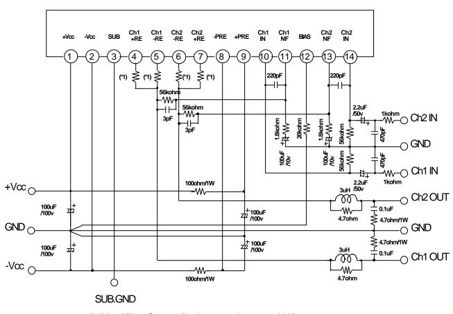
(\*1)Metal Plate Cement Resistor 0.22ohm+10%(5W)
