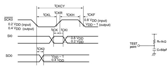
Figure 4 Serial I/O Timing Figure 5
