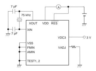
With all ports other than those specified above left open. With output mode selected for PC and PD. With segments S13 to S20 selected.
