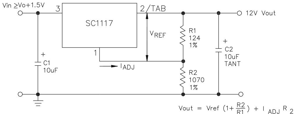
(1) C1 NEEDED IF DEVICE IS FAR FROM FILTER CAPACITORS.
