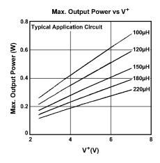
The typical application circuit generates an adjustable negative voltage for contrast bias of LCD displays. Efficiency and output power can be optimized by using the appropriate inductor and switch. The following formulas provide a guideline for determining the optimal component values:
