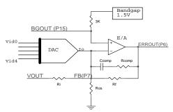
Figure 2: Error amplifier connections
