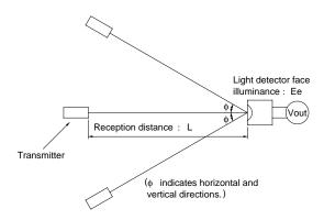
Fig. 2. Standard optical system
