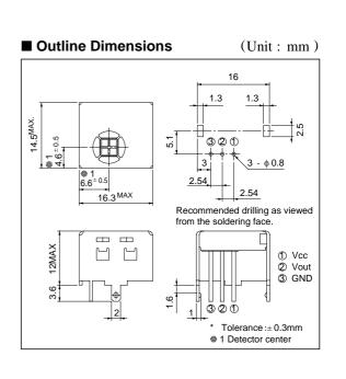
IR Detecting Unit For Remote Control
