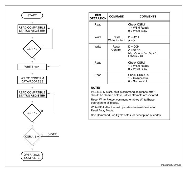
Figure 13. Reset Write Protect
