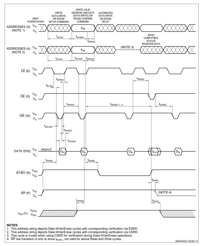
Figure 18. Waveforms for Command Write Operations
