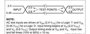
Figure 14. Transient Input/Output Reference Waveform (V<sub>CC</sub> = 5.0 V)
