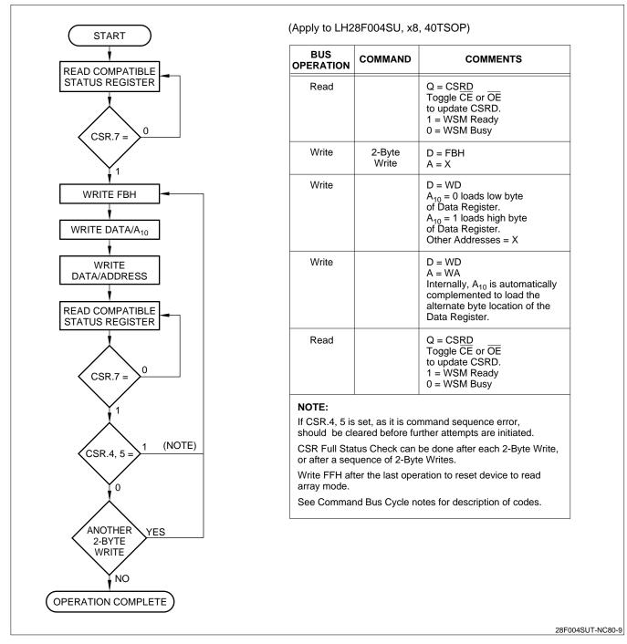
Figure 10. Two-Byte SerialWrites with Compatible Status Registers (LH28F00SU)
