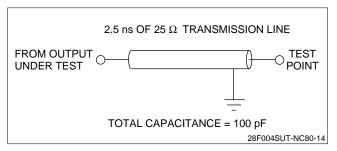
Figure 15. Transient Equivalent Testing Load Circuit (V<sub>CC</sub> = 5.0 V)
