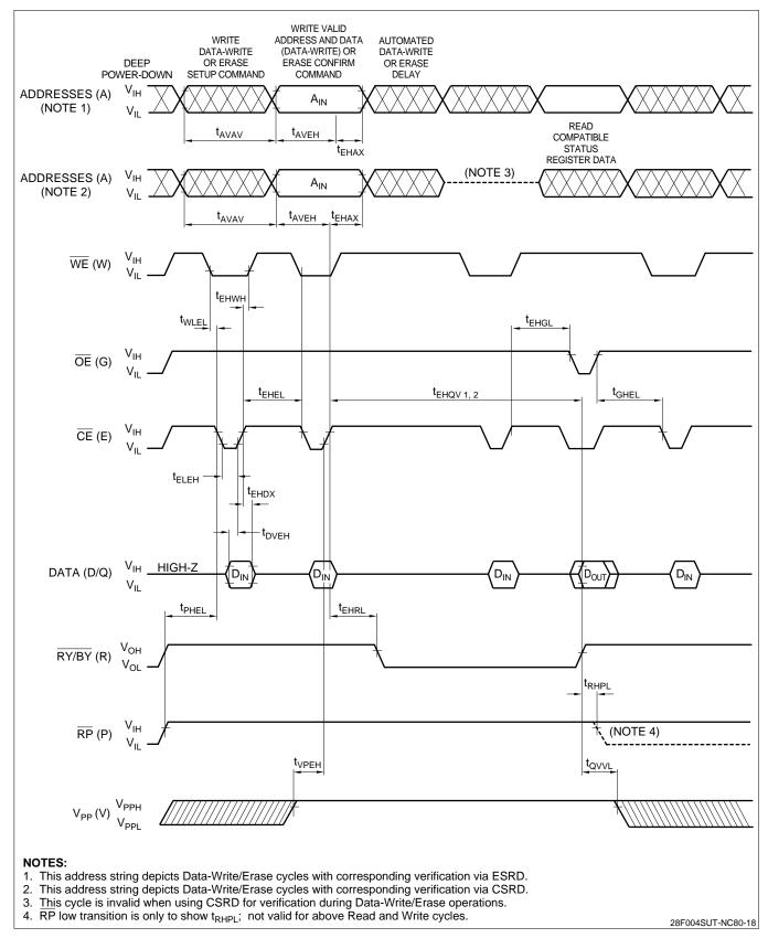
Figure 19. Alternate AC Waveforms for Command Write Operations
