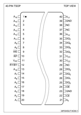
Figure 1. TSOP Configuration
