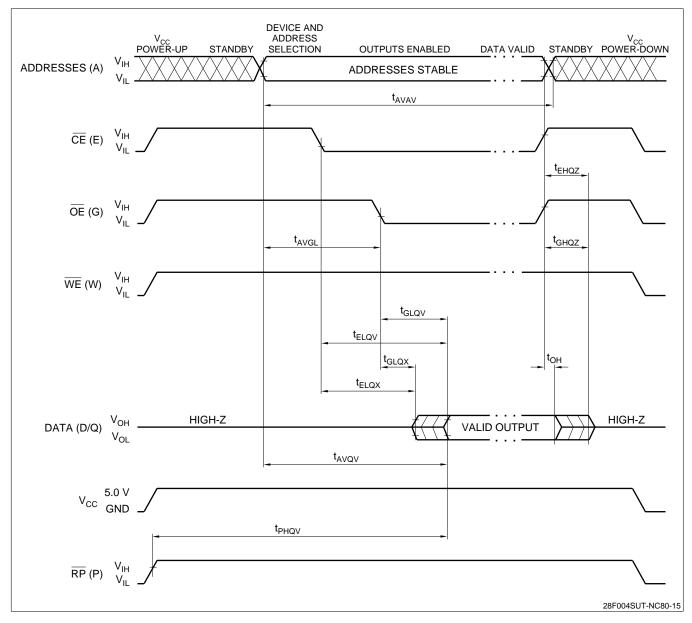
Figure 16. Read Timing Waveforms
