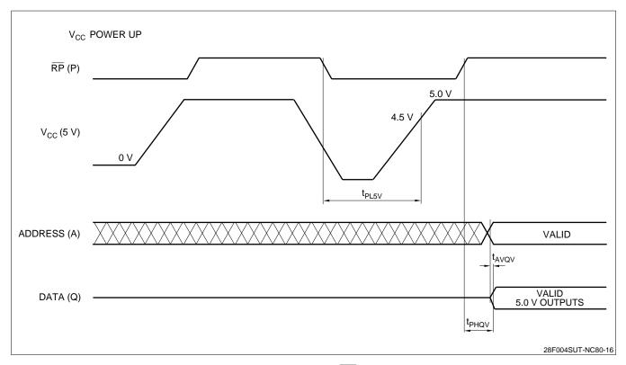
Figure 17.  $V_{CC}$  Power-Up and  $\overline{RP}$  Reset Waveforms
