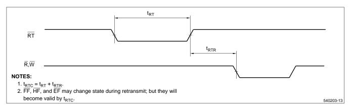
Figure 19. Retransmit Timing
