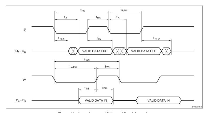
Figure 11. Asynchronous Write and Read Operation
