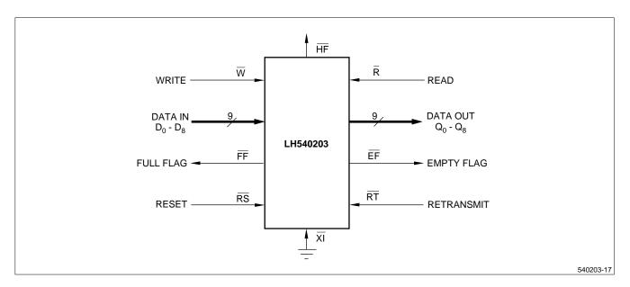
Figure 4. Standalone FIFO (2048  $\times$  9)
