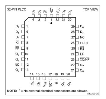
Figure 2. Pin Connections for PLCC Package
