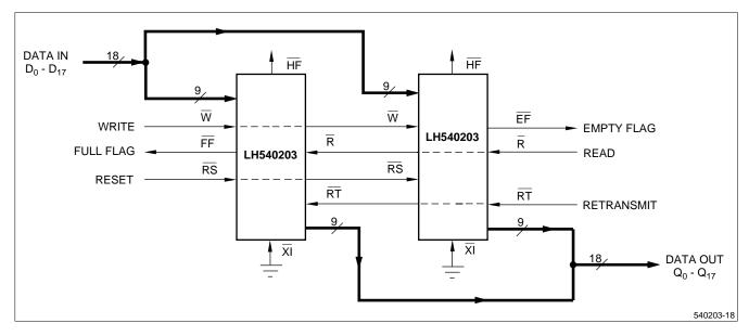
Figure 5. FIFO Word-Width Expansion (2048 × 18)
