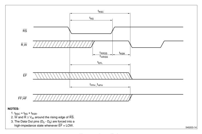
Figure 10. Reset Timing
