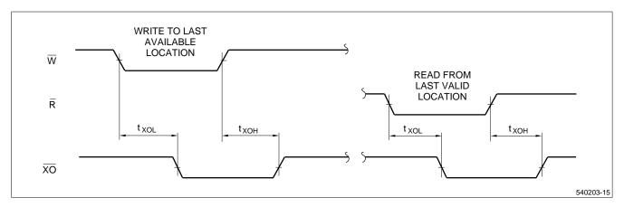
Figure 20. Expansion-Out Timing
