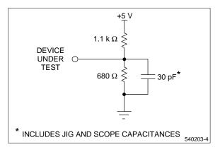
Figure 9. Output Load Circuit
