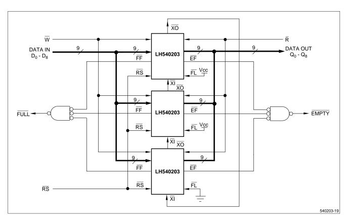
Figure 6. FIFO Depth Cascading ( $6144 \times 9$ )
