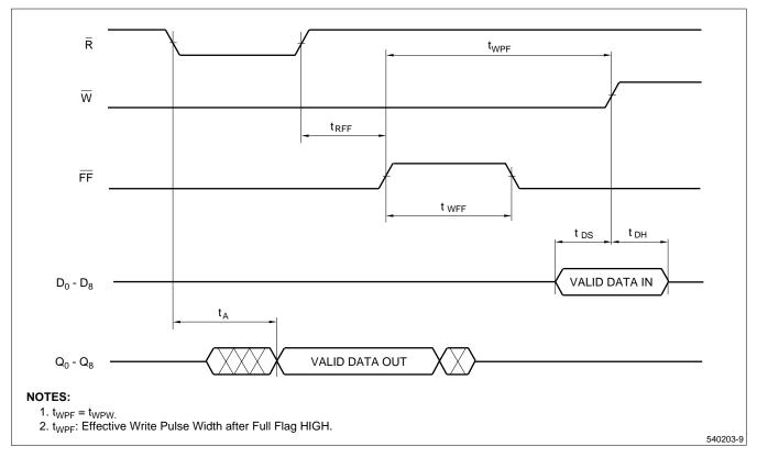
Figure 15. Write Data Flow-Through
