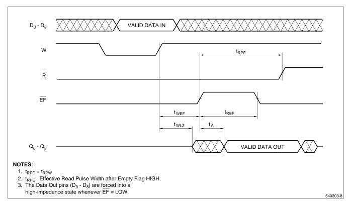
Figure 14. Read Data Flow-Through
