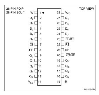
Figure 1. Pin Connections for PDIP and SOJ \* Packages
