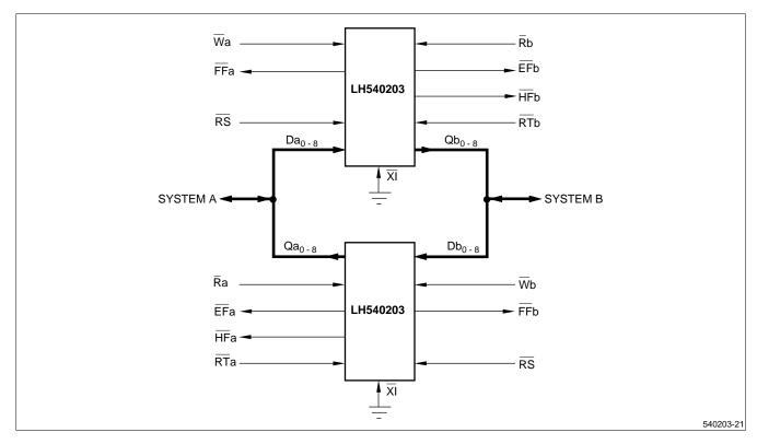
Figure 8. Bidirectional FIFO Operation  $(2048 \times 9 \times 2)$
