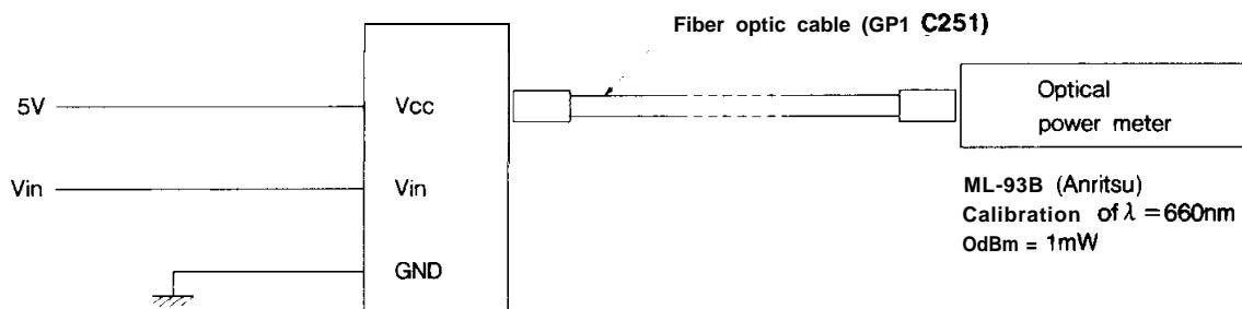
**Fig. 2 Measuring Method (Receiver Unit)**
