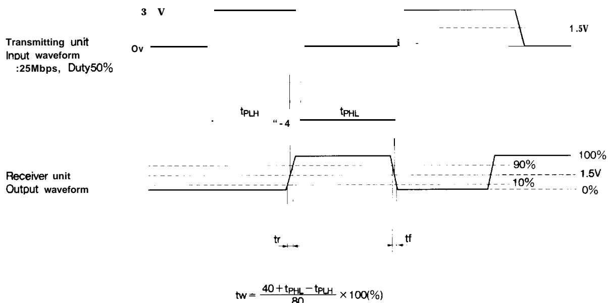
**Fig. 4 Measuring Method (Optical Power Output Coupling with Fiber)**
