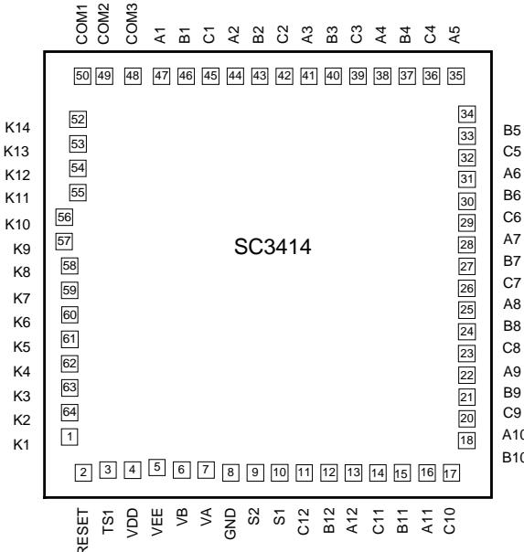
Note: The IC substrate should be connected to GND in the PCB layout artwork.
