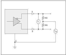
Figure 3. V.35 Driver Output Offset Voltage
