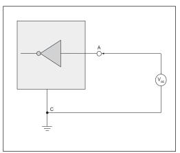
Figure 19. V.28 Receiver Input Open Circuit Bias
