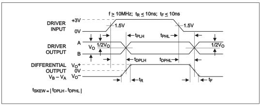
Figure 10. Driver Propagation Delays
