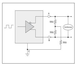
Figure 6. V.35 Driver Output Rise/Fall Time
