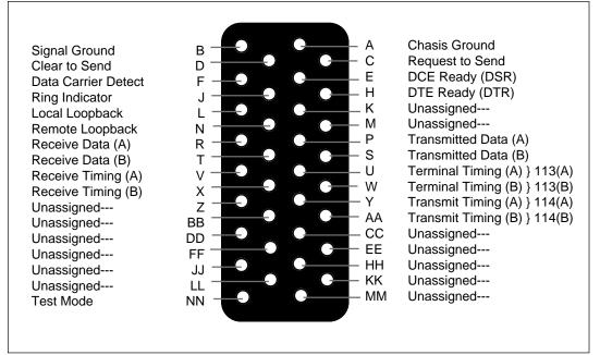
Figure 26. ISO-2593 Connector Pin Out
