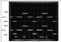
Figure 20. Charge Pump Waveforms
