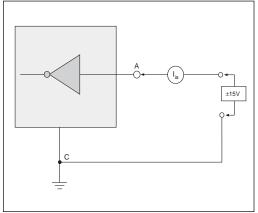
Figure 18. V.28 Receiver Input Impedance
