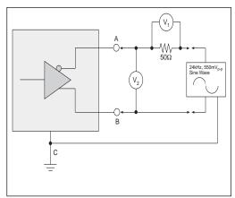
Figure 4. V.35 Driver Output Source Impedance
