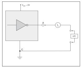
Figure 16. V.28 Driver Output Power-Off Impedance
