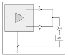
Figure 5. V.35 Driver Output Short-Circuit Impedance
