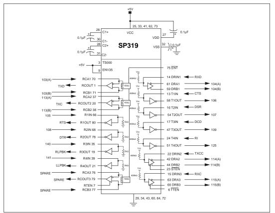
Figure 27. Typical DCE V.35 Interface
