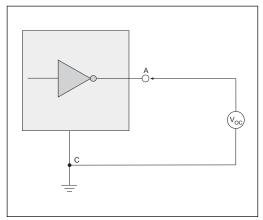
Figure 12. V.28 Driver Output Open Circuit Voltage
