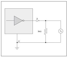
Figure 13. V.28 Driver Output Loaded Voltage
