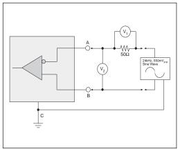
Figure 7. V.35 Receiver Input Source Impedance
