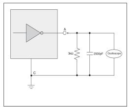
Figure 17. V.28 Driver Output Rise/Fall Times
