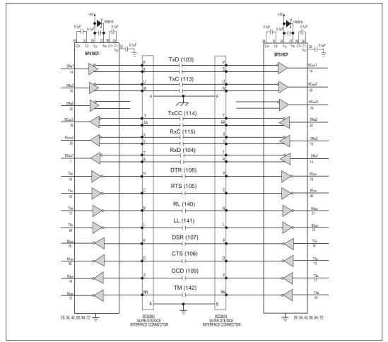
Figure 25. Typical DTE-DCE V.35 Connection using the SP319
