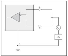
Figure 8. V.35 Receiver Input Short-Circuit Impedance
