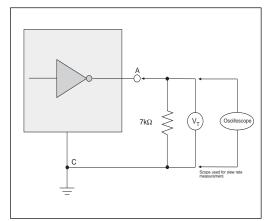
Figure 14. V.28 Driver Output Slew Rate
