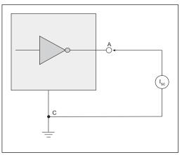
Figure 15. V.28 Driver Output Short-Circuit Current
