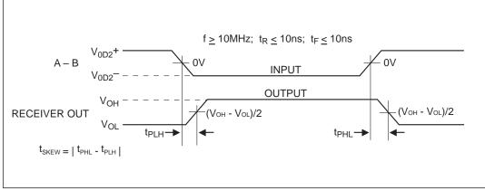
Figure 11. Receiver Propagation Delays
