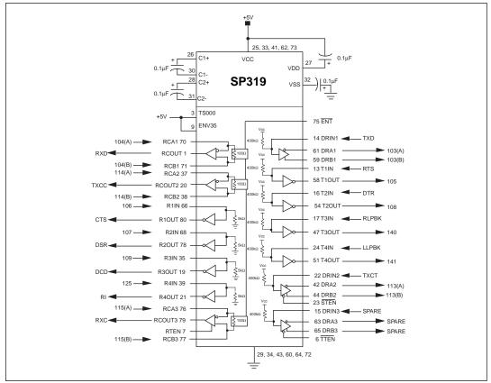
Figure 28. Typical DTE V.35 Interface
