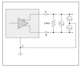
Figure 1. V.11 and V.35 Driver Output Open-Circuit Voltage
