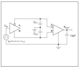
Figure 9. Driver/Receiver Timing Test Circuit
