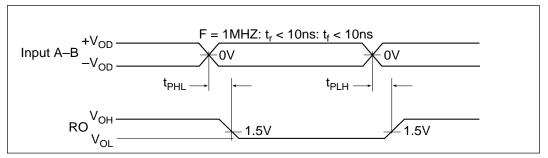
Figure 3. Receiver Propagation Delays
