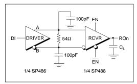
Figure 1. Timing Test Circuit
