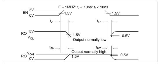
Figure 4. Receiver Enable/Disable Timing
