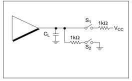
Figure 2. Enable/Disable Timing Test Circuit
