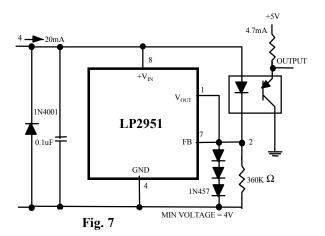
Open Circuit Detector for 4mA to 20mA Current Loop
