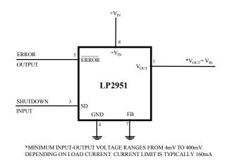
Fig.3 Wide Input Voltage Range Current Limiter
