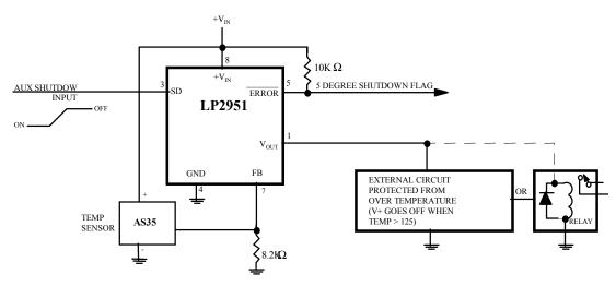
Fig 6. System Over Temperature Protection
