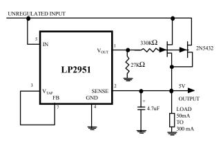
Fig 8. 300 mA Regulator with 0.75V
