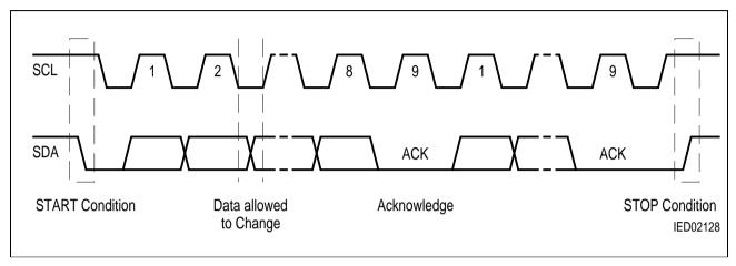
Figure 4  $I^2\text{C-Bus}$  Timing Conventions for START Condition, STOP Condition, Data Validation and Transfer of Acknowledge ACK
