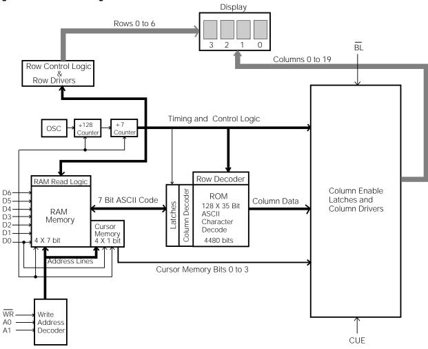
Figure 6. Typica schematic—16-character system
