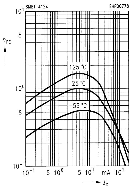
**Small-signal current gain  $h_{fe} = f(I_c)$**
