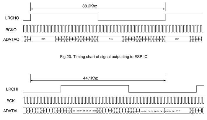
Fig.21. Timing chart of signal ESP IC outputting to DSP
