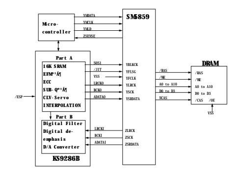
Fig.19. ESP interface application
