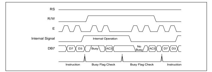
Figure 12. Example of 4-bit Bus Mode Timing Sequence
