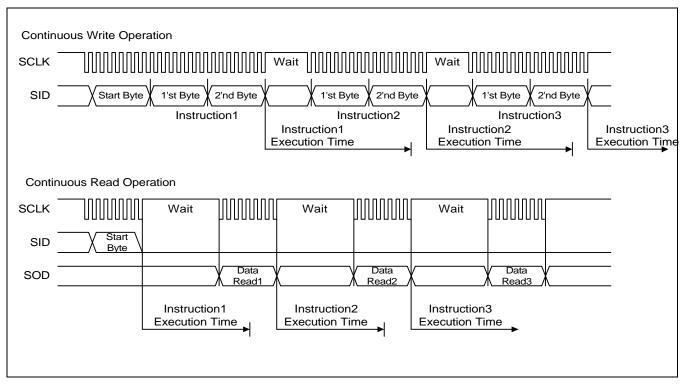
Figure 14. Timing Diagram of Continuous Data Transfer
