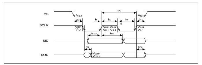
Figure 17. Serial Interface Mode
