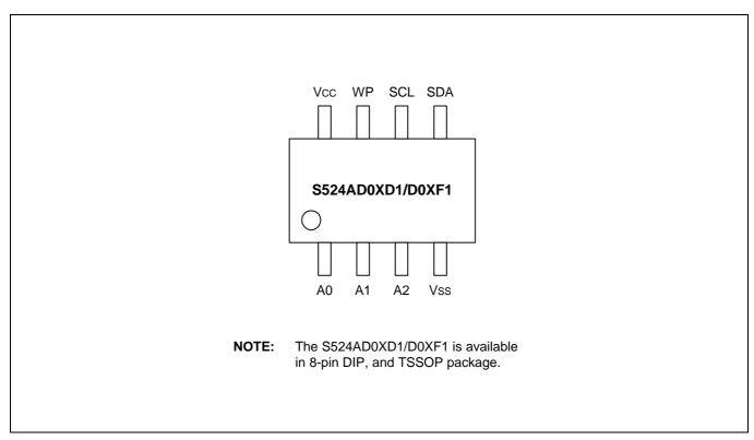
Figure 8-2. Pin Assignment Diagram
