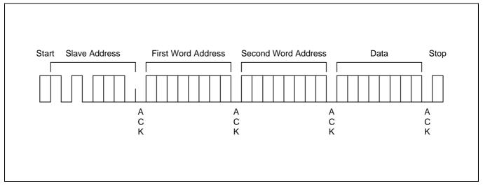
Figure 8-10. Byte Write Operation
