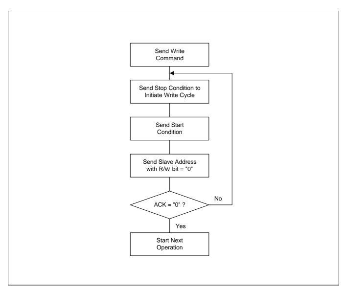
Figure 8-12. Master Polling for an ACK Signal from a Slave Device
