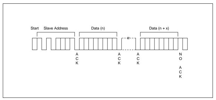
Figure 8-15. Sequential Read Operation
