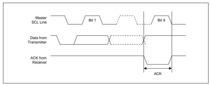
Figure 8-8. Acknowledge Response from Receiver
