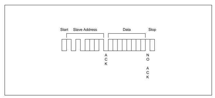
Figure 8-13. Current Address Byte Read Operation
