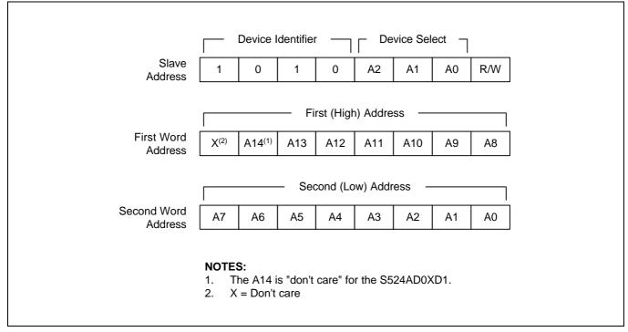
Figure 8-9. Device Address
