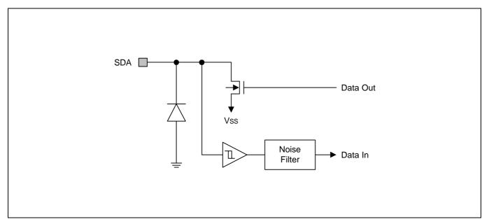
Figure 8-5. Pin Circuit Type 3
