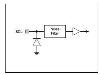
Figure 8-3. Pin Circuit Type 1
