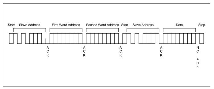
Figure 8-14. Random Address Byte Read Operation
