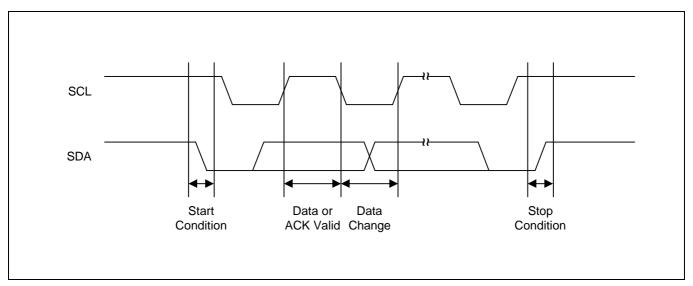
Figure 8-7. Data Transmission Sequence
