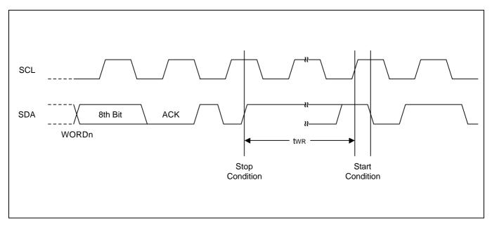
Figure 8-17. Write Cycle Timing Diagram
