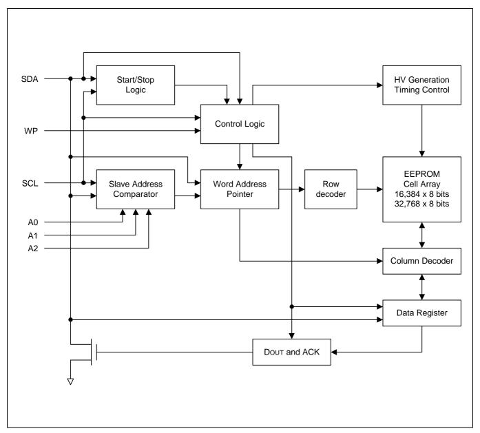
Figure 8-1. S524AD0XD1/D0XF1 Block Diagram
