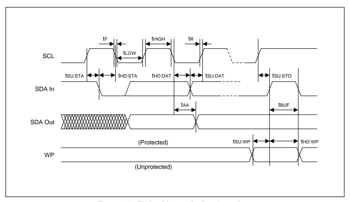
Figure 8-16. Timing Diagram for Bus Operations
