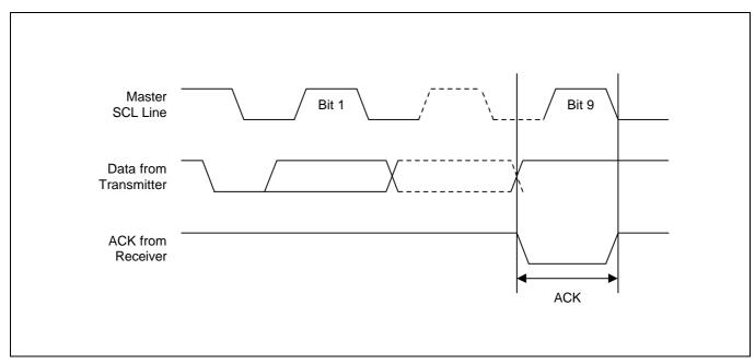
Figure 4-8. Acknowledge Response From Receiver
