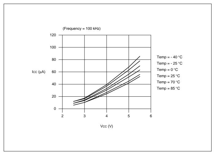
Figure 4-19. I<sub>CC</sub> (Read Current) vs. V<sub>CC</sub>
