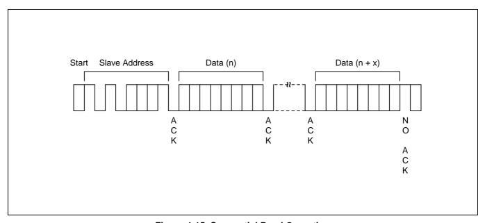
Figure 4-15. Sequential Read Operation
