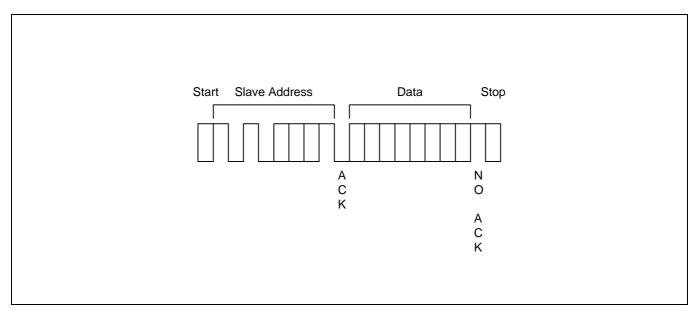
Figure 4-13. Current Address Byte Read Operation
