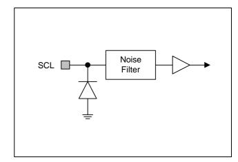
Figure 4-3. Pin Circuit Type 1
