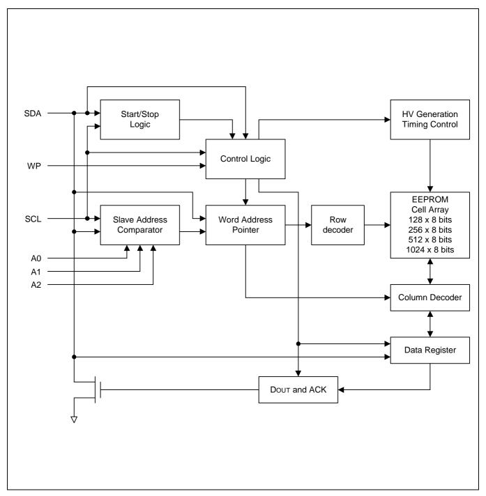
Figure 4-1. S524C20D10/20D20/80D40/80D80 Block Diagram
