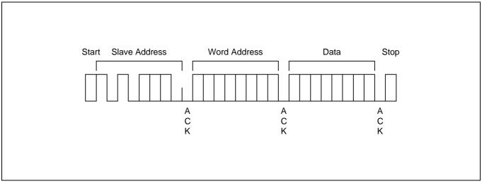
Figure 4-9. Byte Write Operation
