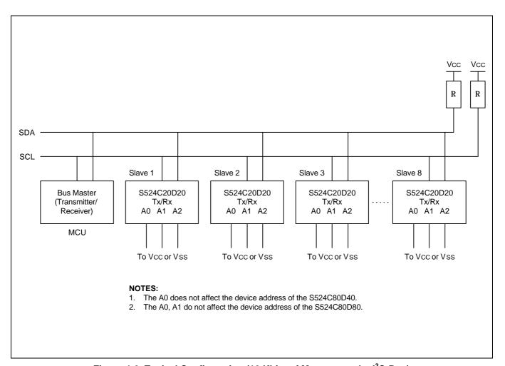
Figure 4-6. Typical Configuration (16 Kbits of Memory on the I<sup>2</sup>C-Bus)
