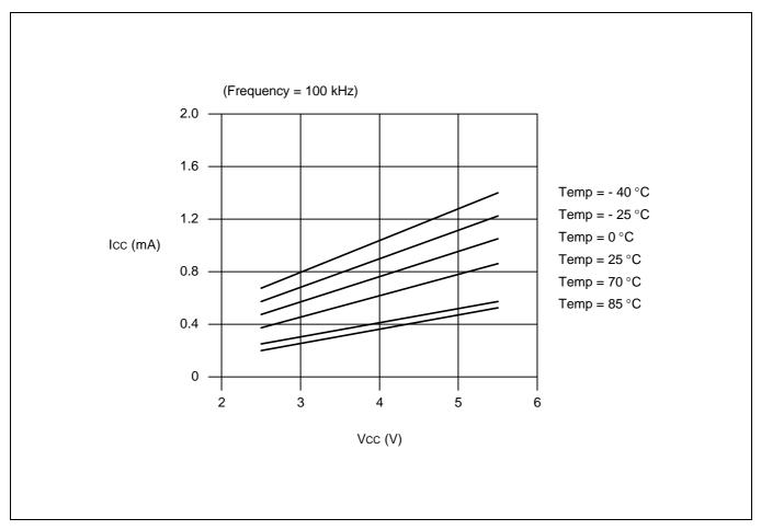
Figure 4-18.  $I_{CC}$  (Write Current) vs.  $V_{CC}$
