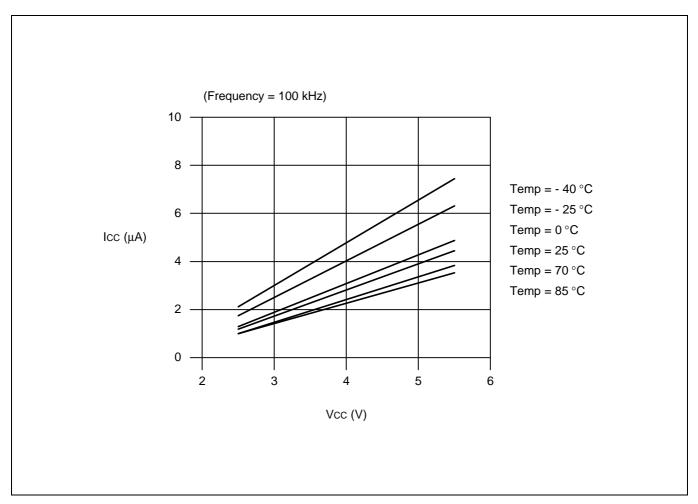
Figure 4-20.  $I_{CC}$  (Stand-by Current) vs.  $V_{CC}$
