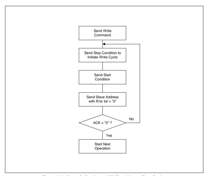
Figure 4-11. Master Polling for an ACK Signal from a Slave Device
