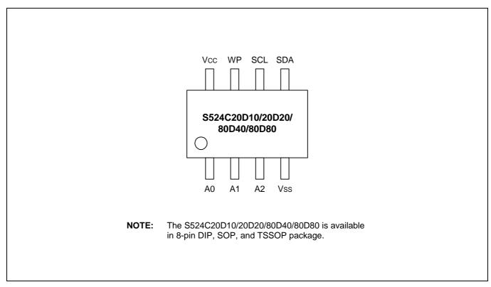
Figure 4-2. Pin Assignment Diagram
