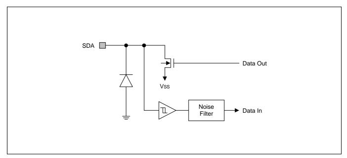
Figure 4-5. Pin Circuit Type 3
