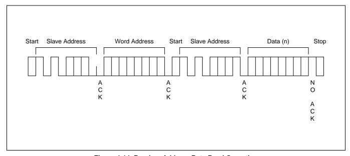
Figure 4-14. Random Address Byte Read Operation
