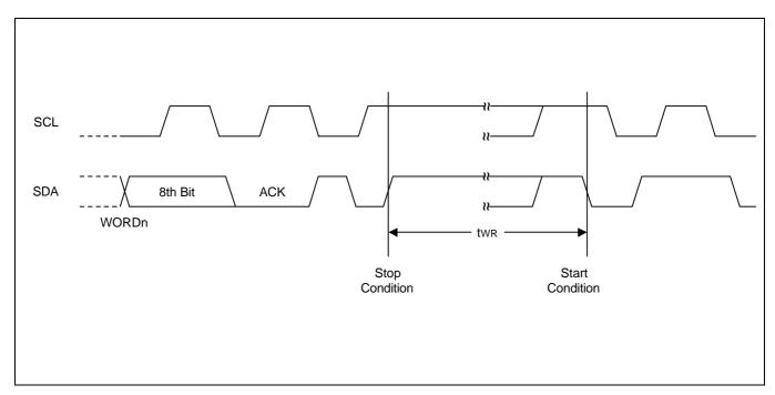
Figure 4-17. Write Cycle Timing Diagram
