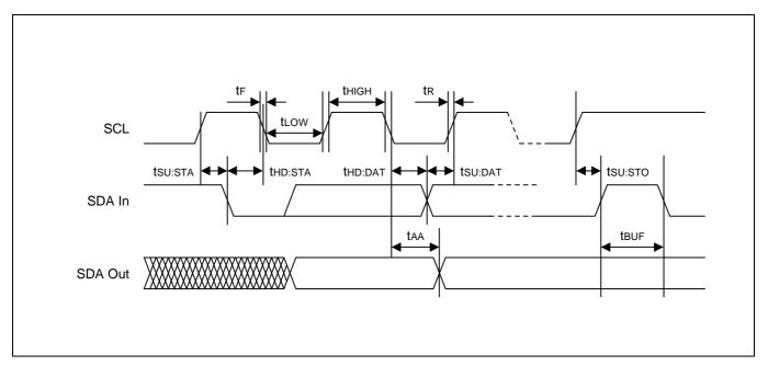
Figure 4-16. Timing Diagram for Bus Operations
