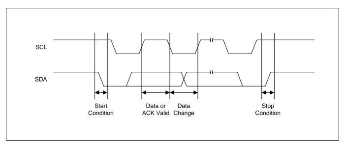
Figure 4-7. Data Transmission Sequence
