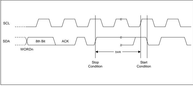
Figure 5-16. Write Cycle Timing Diagram
