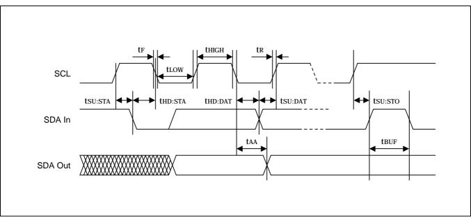
Figure 5-15. Timing Diagram for Bus Operations
