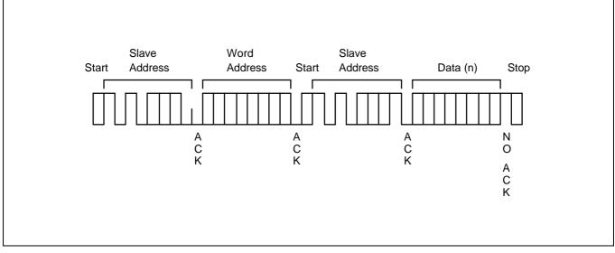
Figure 5-13. Random Address Byte Read Operation
