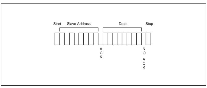
Figure 5-12. Current Address Byte Read Operation
