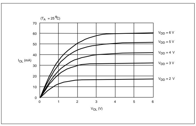
Figure 5-20. Output Low Voltage
