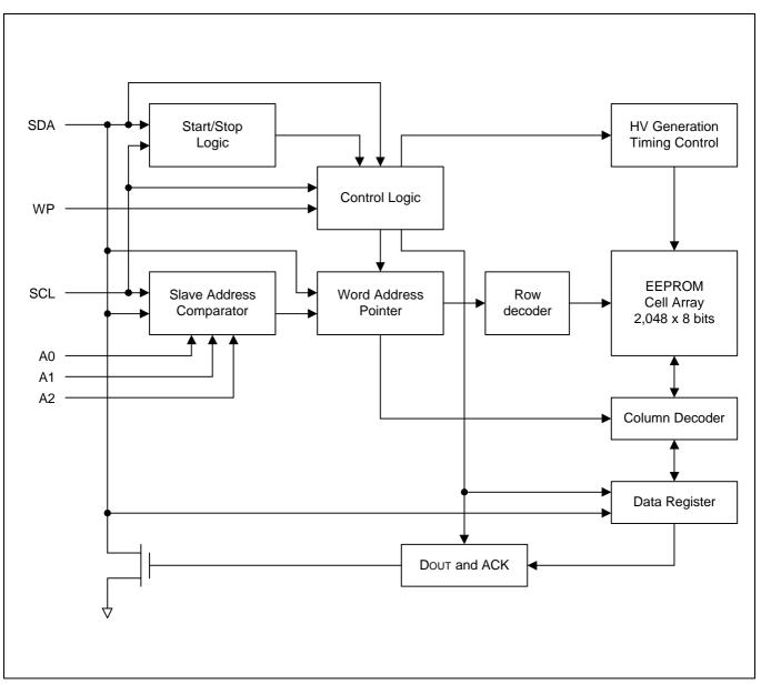
Figure 5-1. S524L50X51 Block Diagram
