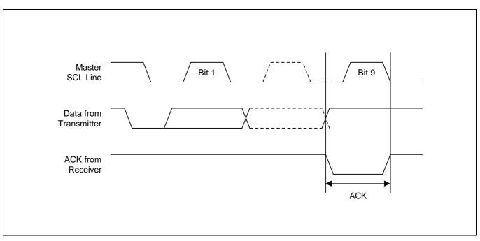
Figure 5-8. Acknowledge Response From Receiver
