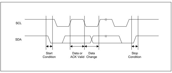
Figure 5-7. Data Transmission Sequence
