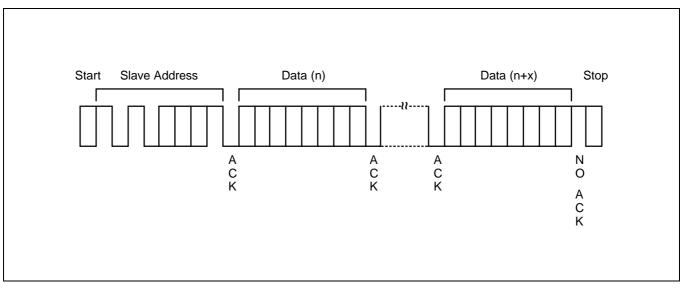
Figure 5-14. Sequential Read Operation
