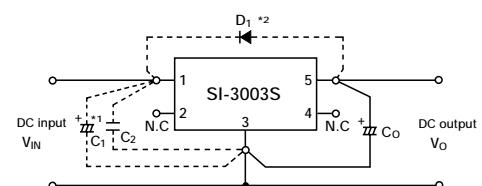
C<sub>O</sub> : Output capacitor (47 to 100μF, 50V)
