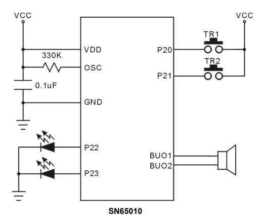
Note: Please bonds all of  $V_{\text{DD}}$  and  $V_{\text{SS}}$  pins.
