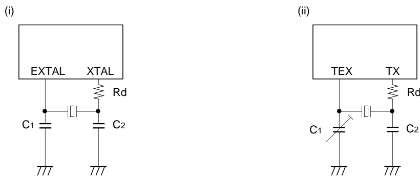
Fig. 11. SPC700 Series recommended oscillation circuit
