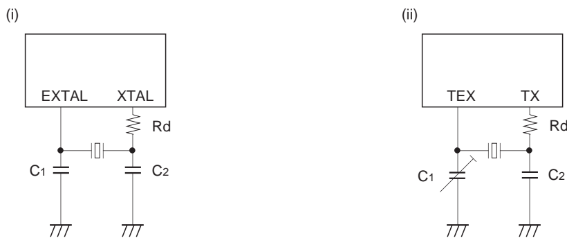
Fig. 13. Recommended oscillation circuit
