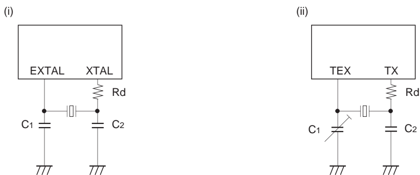
Fig. 9. Recommended oscillation circuit
