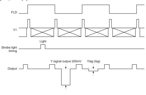
Drive Circuit 1 (substrate bias internal generation mode)
