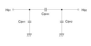
Vertical transfer clock equivalent circuit
