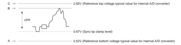
The DC level at the ADIN pin is as shown in the diagram above when the internal sync tip clamp is used.
